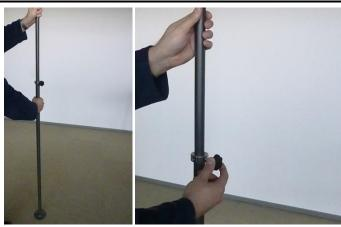
4. Mount the bottom part of the telescope in the foot socket, by pressing it and turning it by 90°, and then locking the support by spring in the foot socket. Then tighten the telescope knob until resistance is felt.
