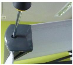
3. Unscrew the fastening screws at both ends of the front bar and remove the end caps by pushing them outside.
