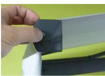
6. Install and tighten the end caps. Put on the screw covers.
